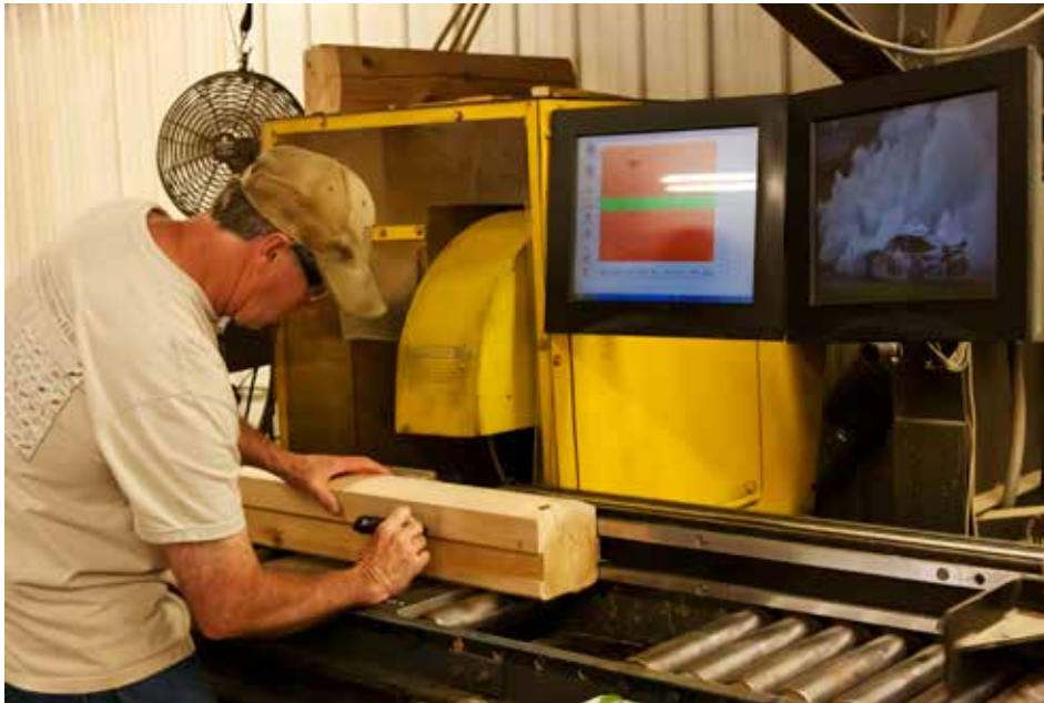
Log home line operator Wendell Hersey feeds planed wood through for finishing. The manufacturing line operates through a computer that reads the home design plans and makes precise, laser-guided cuts for each log in the kit.
