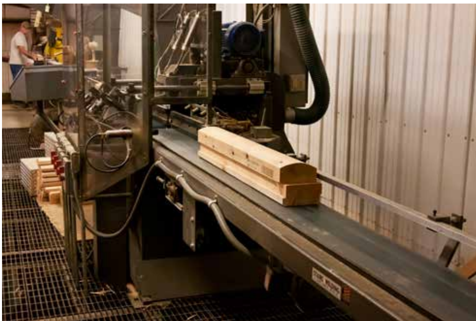
Each log is stamped with an identifying barcode and letter/number corresponding to its location on the home plan and then stacked in reverse order on pallets to be shipped to the builder.
